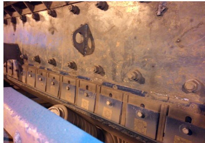
Segmented skirt sealing previously used
