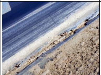
The damage was caused by age and running material with excessive weight over a belt with an idler configuration designed to handle a lighter load.
